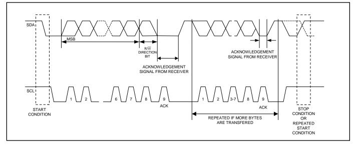
Depending upon the state of the R/w bit, two types of data transfer are possible:
